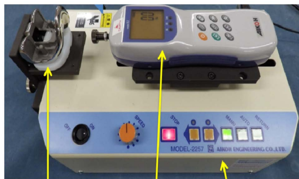
Knee Prosthesis (Polyethylene insert) Force Gauge Compression Tester
