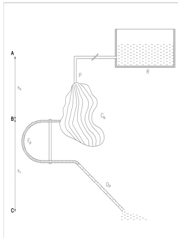
**Figure 2.** Simple sketch of the novel pulsatile flow generator. R is reservoir; P are connecting pipes from reservoir to collapsing bladder  $C_b$ . The collapsible bladder is connected to ‘U’ shaped flexible tube  $F_p$  which is in turn connected to long rigid distal pipe  $D_p$ .
