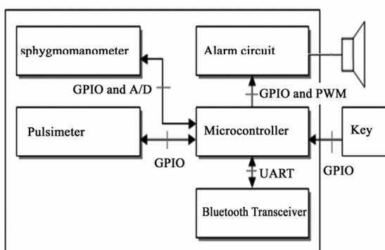
**Figure 2.** Wristable sphygmomanometer and pulsometer hardware architecture.
