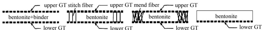
**Figure 1.** Sketch of four basic GCLs products.
