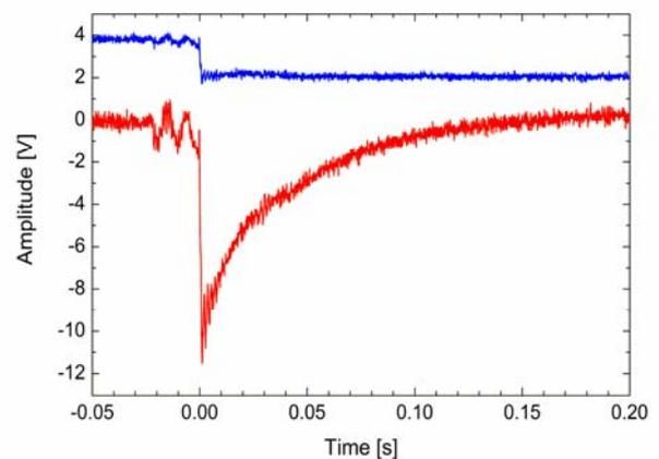
**Figure 3.** The output signal of the oscillometric amplifier (lower curve) as a response to a step-like change in its input (upper curve); the latter has been multiplied by a factor of 50, and displaced vertically in order to bring it within the frame.
