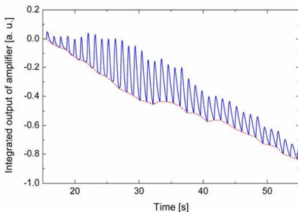
**Figure 5.** Plots of  $N(t)$ , the integral of the amplifier output (continuous curve) and  $L(t)$ , the baseline (dotted curve) obtained by passing a continuous curve through the minima of  $N(t)$ .
