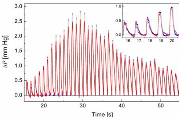
**Figure 6.** Plots of the pulsating part of the cuff signal (continuous curve) and the integral of the amplifier output signal after baseline subtraction (open circles). The inset shows the early part of the deflation phase (where the deviation between the two curves is most pronounced).
