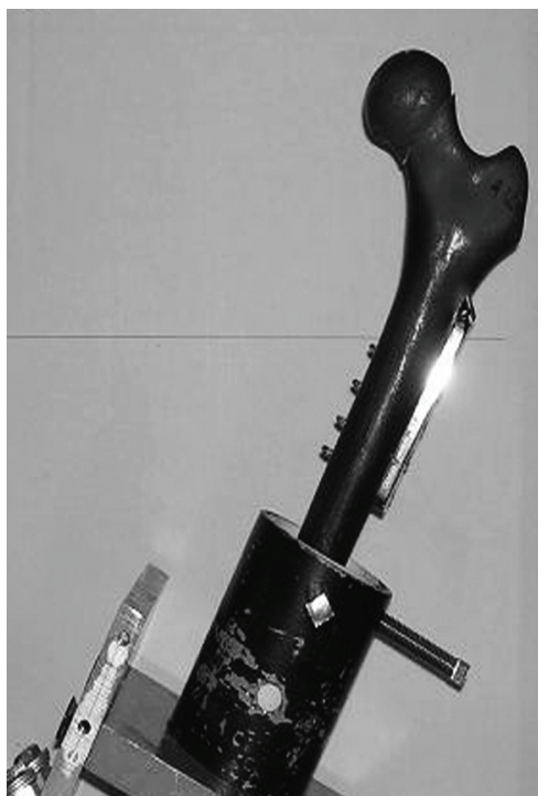
Figure 4. Testing jig used for mechanical testing of constructs.
