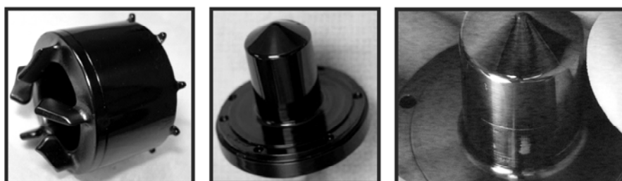
Figure 4. BMF-coated RVAD RA (left) and stator assembly (middle); commercial DLC-coated stator assembly scratches post-test (right).
