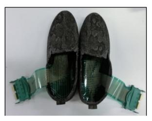
Figure 3. The in-shoe pressure system (Pressure sensor).
