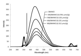
Figure 2. Fluorescence spectra of solutions of MB in BMIMCl in various concentrations excited at 350 nm.
