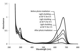
Figure 1. UV-Vis spectra of a solution of MB in BMIMCI before and after photo irradiation (12 h), and spectra of the solution which was left further standing under the conditions of light shielding at 50°C for 2, 4, and 6 h.
