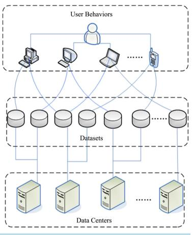
Figure 1. Physical model of data scheduling between data center.
