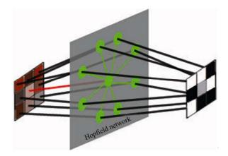
Figure 3. Every  $1^{st}$  layer minicolumn tries to change local images into binary texture patterns, for a  $3 \times 3$  small window, a minicolumn in the  $1^{st}$  layer contains 9 Hopfield neurons, and every neuron focuses only one pixel.
