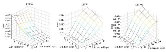
Figure 9. Rmse affected by\_in first layer and second layer, we set Threshold in Equation (1.17) = 1.6.
