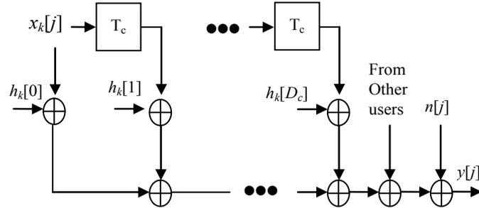
Figure 2. The multipath channel model, where  $D_c$  is the number of paths.
