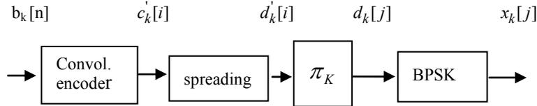
Figure 1. The transmitter model for user  $k$ .
