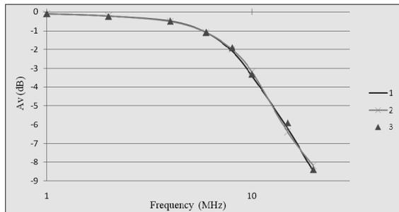
Figure 13. Filter frequency responses in three samples.
