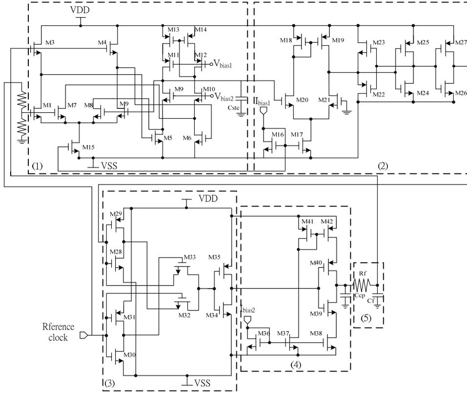
**Figure 7. The structure of proposed tuning circuit ((1): STC circuit, (2): Voltage comparator, (3): Phase Detector, (4): Charge Pump, (5): Low Pass Filter).**
