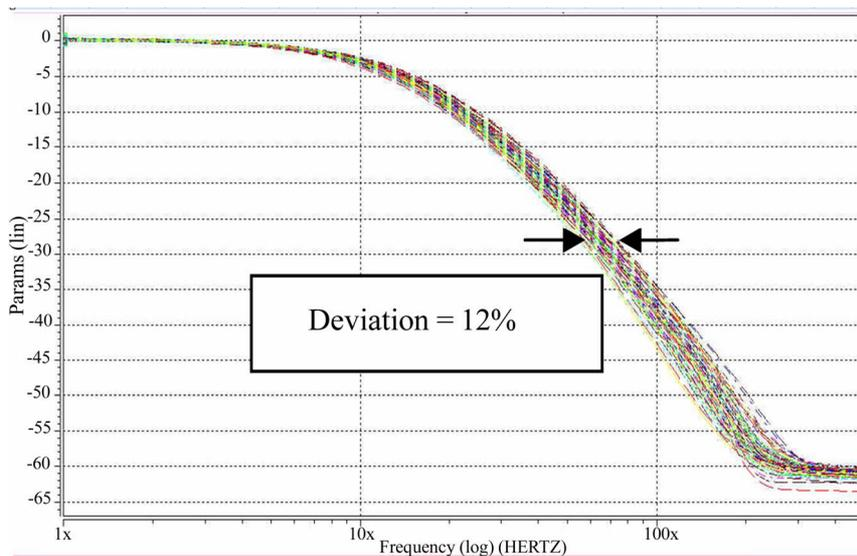
Figure 10. The 3-dB frequency variation in sixty corners (with tuning).
