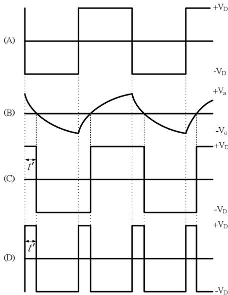
**Figure 4. (A) Reference clock (B) The output of the STC circuit (C) The output of the voltage comparator (D) The output of the PD.**
