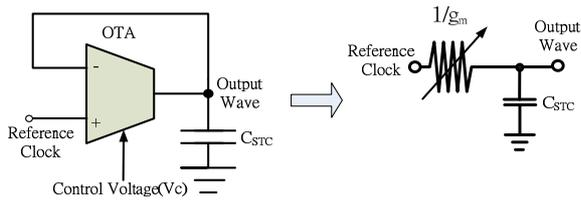
**Figure 2. The STC circuit.**
