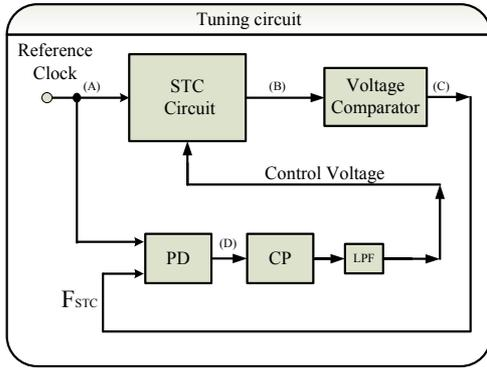
**Figure 1. The block diagram of tuning circuit. (PD: Phase Detector, CP: Charge Pump, LPF: Low Pass Filter).**
