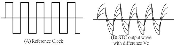
**Figure 3. (A) Reference clock (B) STC output wave with three different Vc.**
