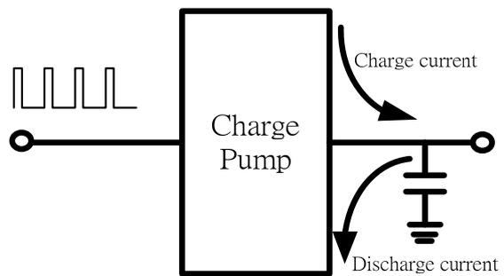
**Figure 6. Charge and discharge current.**
