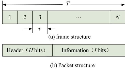
Figure 2. Structure of frame and packet.
