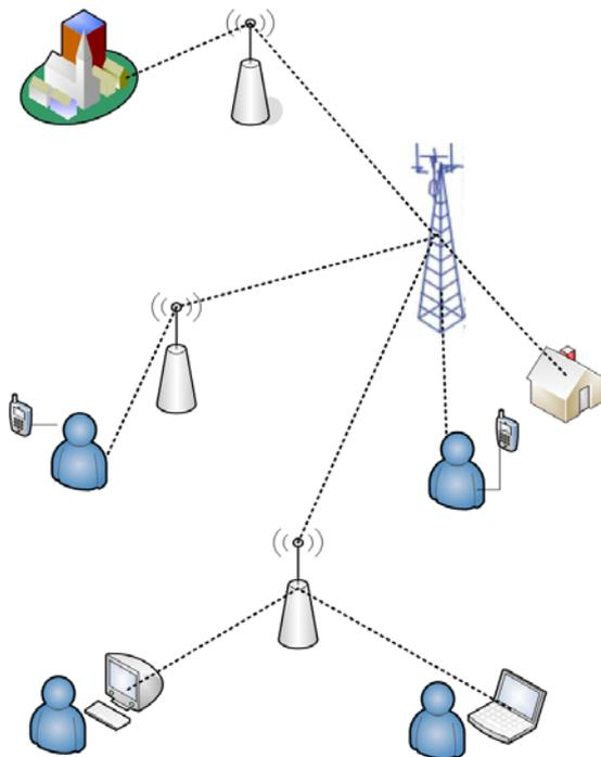
**Figure 1.** Example of a multihop cellular network.
