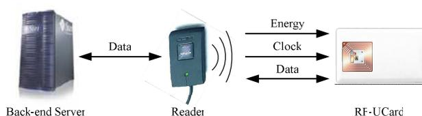
Figure 1. RF-UCard system architecture.
