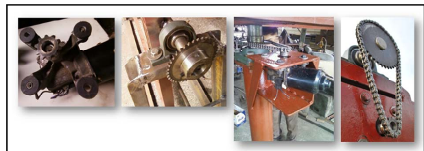
From left to right: Sprocket attached to motor, sprocket attached to frame, chain connecting the two sprockets
