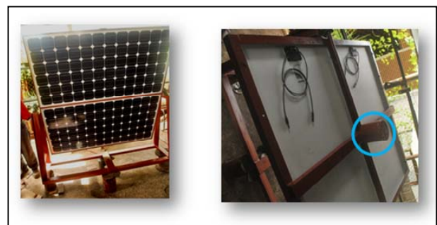
Figure 5. The solar panel affixed to the frame (left). The counter-weight (circled, right).
