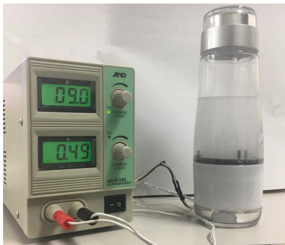
Figure 1. Hydrogen/free chlorine mixed water generator and power supply unit (DC stabilized power supply, A & D Co., Ltd., Japan) used for experiment.
