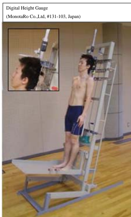
Figure 1. Stadiometer, the apparatus for measuring change in stature.
