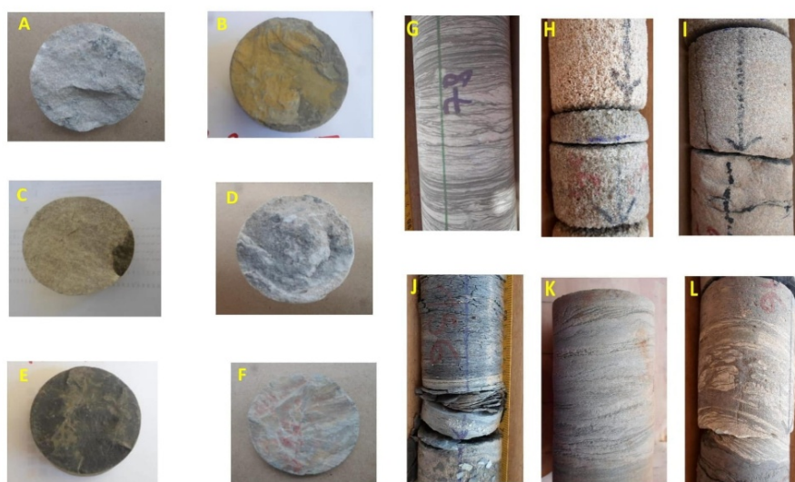
Figure 13. Drill cores samples of Tamari prospect area with yellow to red color and cross-stratification.
