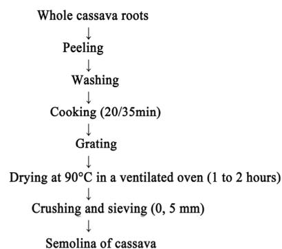
**Figure 1. Diagram of semolina preparation**
