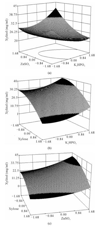
Figure 1. Response surface plot showing the effect of xylose,  $K_2HPO_4$  and  $ZnSO_4$  on xylitol production. (a) Response surface plot showing the effect of  $ZnSO_4$  and  $K_2HPO_4$  on xylitol production at xylose 100 g/l; (b) Response surface plot showing the effect of xylose and  $K_2HPO_4$  on xylitol production at 8.9 mg/l of  $ZnSO_4$ ; (c) Response surface plot showing the effect of ZnSO4 and xylose on xylitol production at 10 g/l of  $K_2HPO_4$ .
