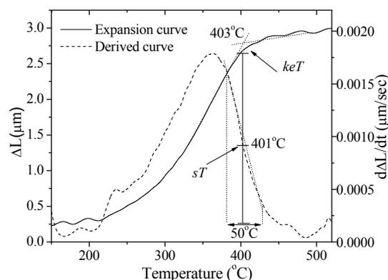
**Figure 5.** Dilatometric curve of the dissolution process and derivative. The arrows indicate the change in the slope, where the dissolution ends ( $keT$ ) and the middle of the step in the derived curve ( $sT$ ). The sample contains 255 wppm-H.
