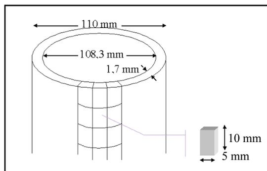
**Figure 1.** Orientation and dimensions of the dilatometric samples.
