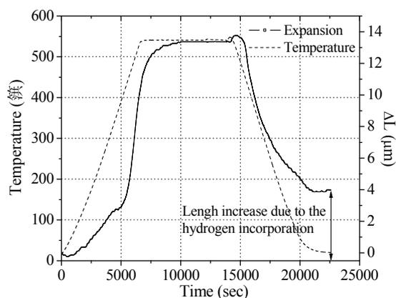
**Figure 4.** Dilatometric thermal cycle to diffuse the hydrogen from the layers into the bulk.
