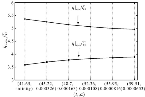
**Figure 16.** The normalized peak tsunami amplitudes  $|\eta|_{\min}/\zeta_0$  and  $|\eta|_{\max}/\zeta_0$  at time  $t = t_{\max}$  for the different deceleration  $\alpha$  and time  $t_3$ .
