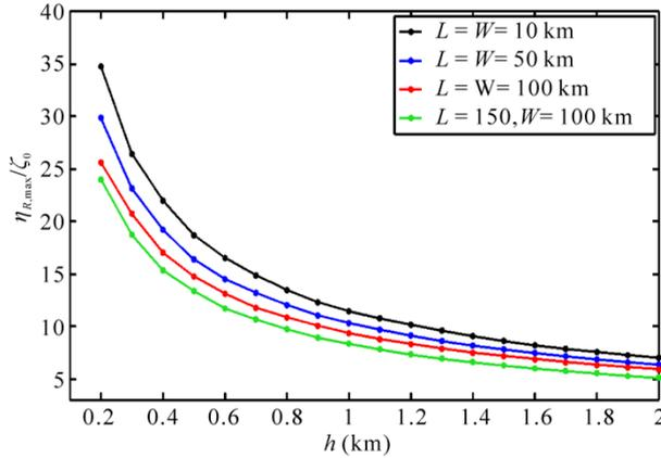
**Figure 12.** Normalized maximum tsunami amplitudes  $\eta_{R,max}/\zeta_0$  when the slide stops suddenly at time  $t_{min} = t^* + (L'/v)$  with different slide lengths  $L$  and widths  $W$  and for  $v = v_t$ .
