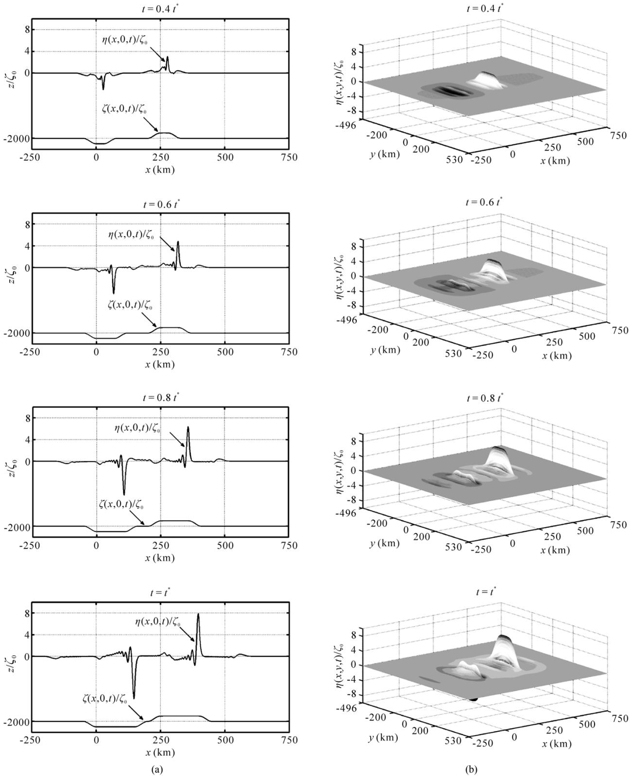
**Figure 6. Dimensionless free-surface elevation caused by the propagation of the slump and slide in the x-direction during the second stage with  $v = v_t$  at  $h = 2$  km,  $L = 150$  km,  $W = 100$  km and  $t^* = 200/v$  sec; (a) Side view along the axis of symmetry at  $y = 0$ ; (b) Three-dimensional view.**
