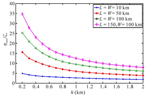
**Figure 9.** Normalized maximum tsunami amplitudes  $\eta_{R,max}/\zeta_0$  for different lengths and widths at  $t = t^* = t_1 + L/v$  for  $v = v_t$ .
