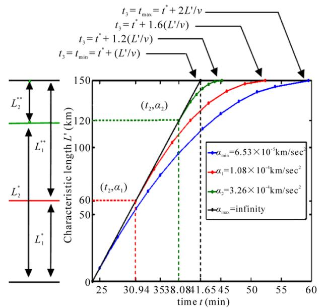
**Figure 5. Slide block position against the instants of times  $t^* \leq t_2 \leq t^* + (L'/v)$  and  $t_{\min} \leq t_3 \leq t_{\max}$ .**
