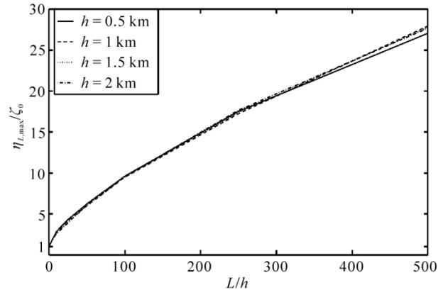
**Figure 8.** Normalized tsunami peak amplitudes,  $|\eta_{L,min}|/\zeta_0$  at the end of second stage for different water depths  $h = 0.5, 1, 1.5$  and  $2$  k at  $t^* = t_1 + L/v$  with  $v = v_t$  and  $L = 150$  km,  $W = 100$  km.
