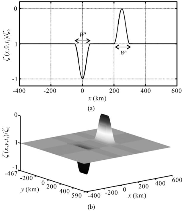
**Figure 2. Normalized bed deformation represented by a rapid curvilinear down and uplift faulting at the end of stage one ( $t_1 = \frac{50}{v}$ ) (a) Side view along the axis of symmetry at  $y = 0$  (b) Three- dimensional view.**
