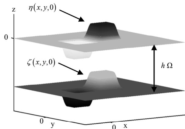
**Figure 1.** Fluid domain and coordinate system for a very rapid movement of the assumed source model.
