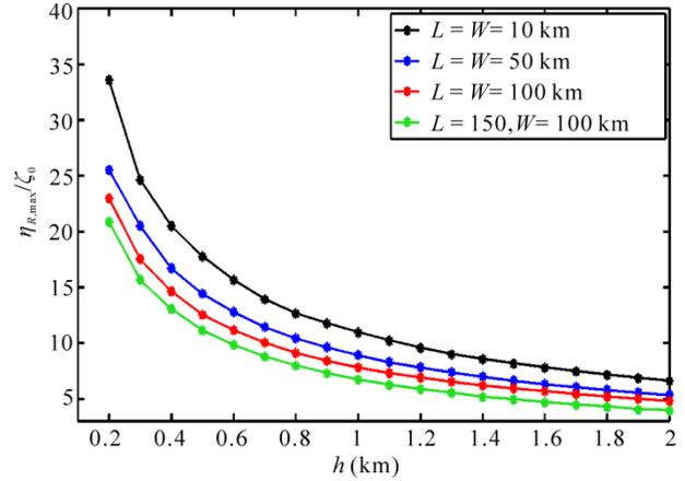
**Figure 13.** Normalized maximum tsunami amplitudes  $\eta_{R,max}/\zeta_0$  when the slide stops softly at time  $t_{max} = t^* + (2L'/v)$  with different slide lengths  $L$  and widths  $W$  and for  $v = v_t$ .
