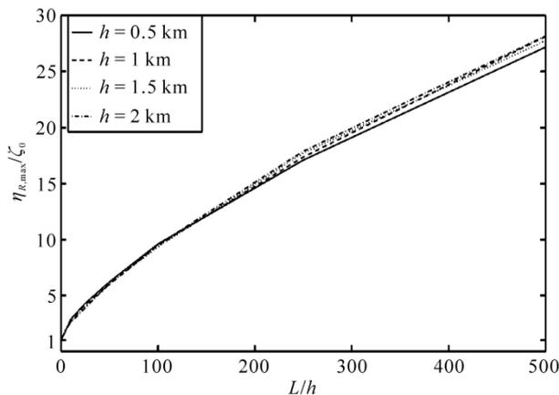
**Figure 7.** Normalized tsunami peak amplitudes,  $\eta_{R,max}/\zeta_0$  at the end of second stage for different water depths  $h = 0.5, 1, 1.5$  and  $2$  k at  $t^* = t_1 + L/v$  with  $v = v_t$  and  $L = 150$  km,  $W = 100$  km.
