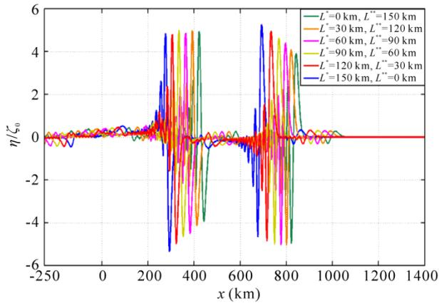
**Figure 14.** Normalized tsunami waveforms  $\eta/\zeta_0$  along  $y = 0$  at  $t = t_3$  calculated in Table 2 with  $L' = 150$  km.
