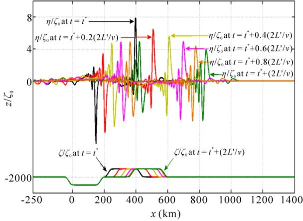
**Figure 11.** Normalized tsunami waveforms  $\eta/\zeta_0$  and their corresponding moving slide  $\zeta/\zeta_0$  with variable velocity  $v(t)$  along  $y = 0$ , at time  $t^* \leq t \leq t^* + (2L'/v)$  at  $h = 2$  km,  $L' = 150$  km and  $W = 100$  km.
