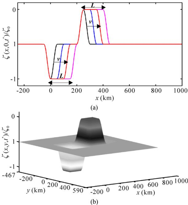
**Figure 3. Normalized Bed deformation model represented by the accumulation and depletion zones at the end of stage two ( $t^* = \frac{200}{v}$ ) (a) Side view along the axis of symmetry at  $y = 0$  (b) Three-dimensional view.**
