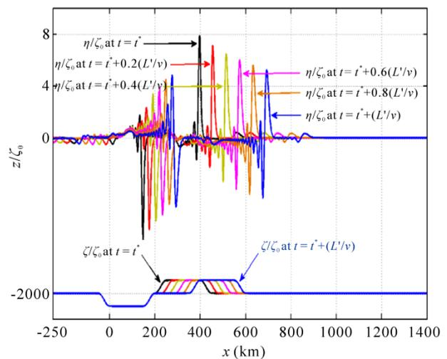
**Figure 10.** Normalized tsunami waveforms  $\eta/\zeta_0$  along the axis of symmetry at  $y = 0$  and their corresponding moving slide  $\zeta/\zeta_0$  with constant velocity  $v$  along  $y = 0$ , at time  $t^* \leq t \leq t^* + (L'/v)$  for  $h = 2$  km,  $L' = 150$  km and  $W = 100$  km.
