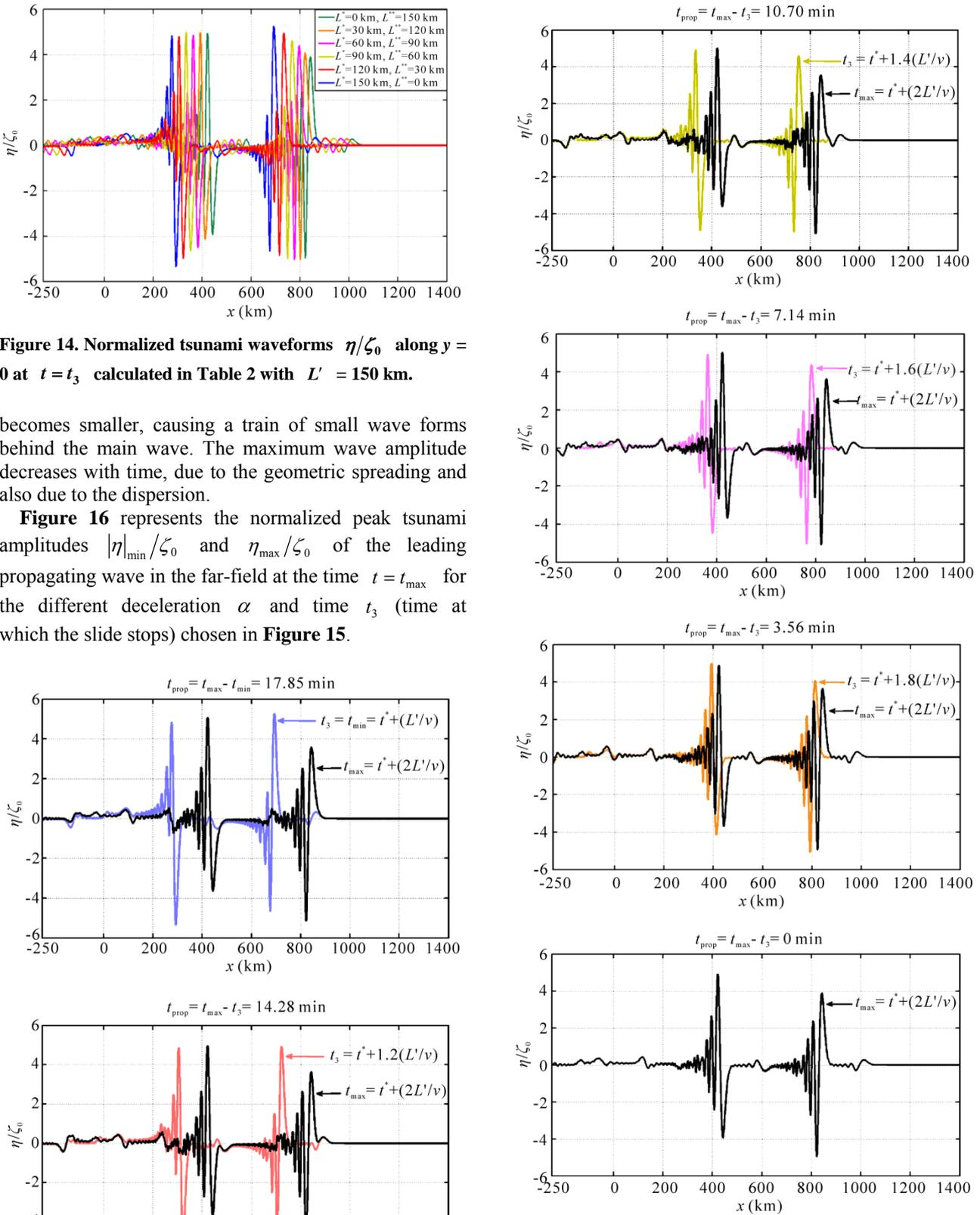
**Figure 15.** Normalized tsunami propagation waveforms  $\eta/\zeta_0$  along the axis of symmetry at  $y = 0$  at time  $t_{\max} = 59.51$  min and at time  $t_3$  for different deceleration  $\alpha$ .
