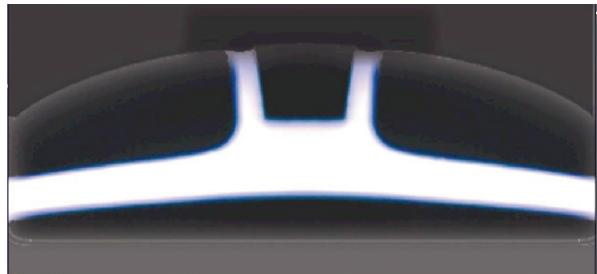
**Figure 1.** Air gap between the electrodes of Enercon plasma treater, occupied by the glowing gas. Gap dimension can range from 1 mm to 2.5 mm. Polymeric films run above the lower electrode connected to the ground.
