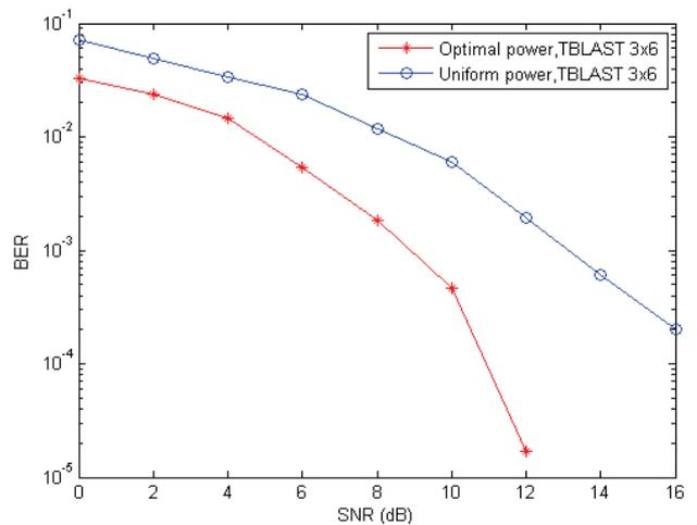
**Figure 3. BER Performance comparison: OPL versus equal power allocation.**
