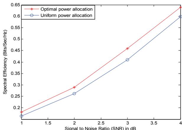
**Figure 4. Comparison of spectral efficiency: OPL versus uniform power allocation.**
