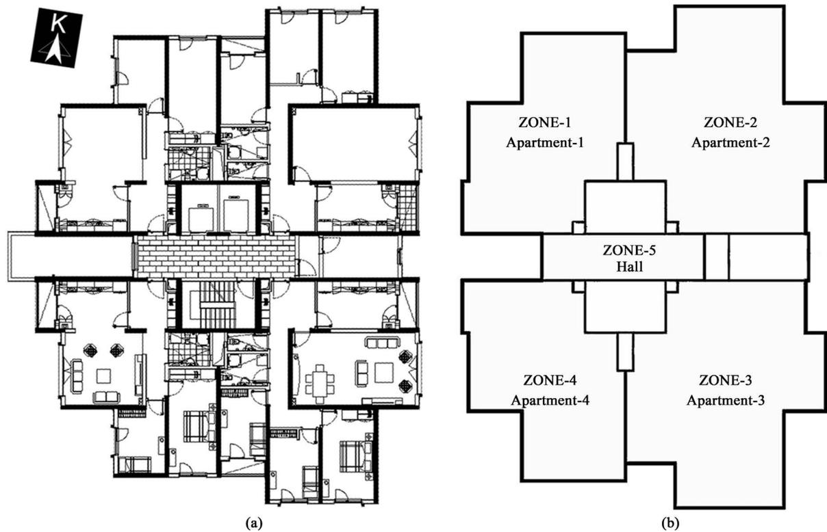
**Figure 2.** (a) Plan view of the reference building and (b) conditioned zone areas.
