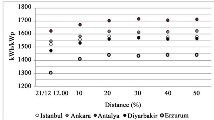
**Figure 5.** The final PV system yield related to the row distance.
