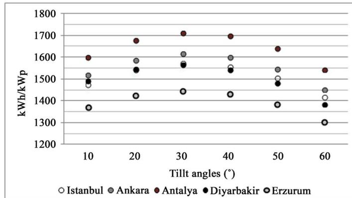
**Figure 4.** The final PV system yield related to the different tilt angles.
