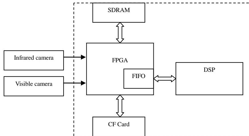
**Figure 1.** Embedded image processing system based on DSP + FPGA.
