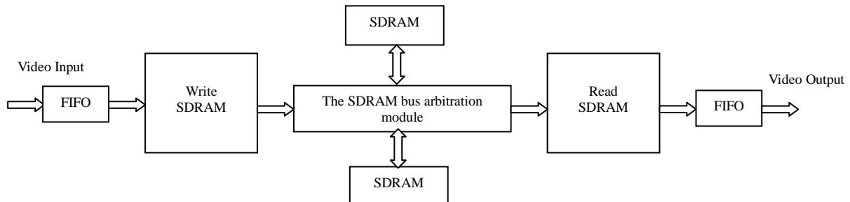
**Figure 4.** Pong operation procedures schematic.
