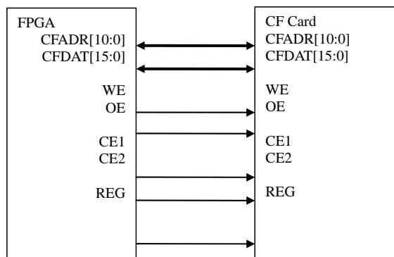
**Figure 3.** The hardware interface between FPGA and CF card.
