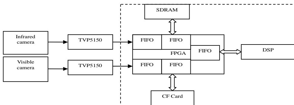
**Figure 2.** The structure diagram of video data acquisition and storage.
