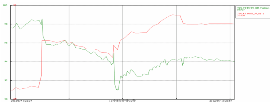
Figure 4. Power generation load and hydroelectric generating efficiency curve.
