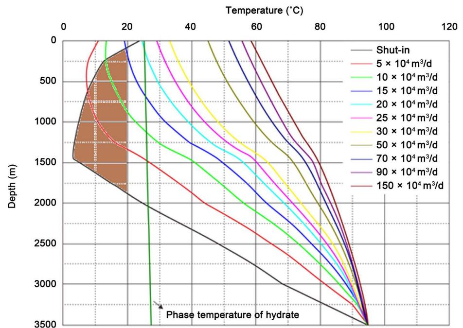
**Figure 2.** Generated area of hydrate under different flow capacity.
