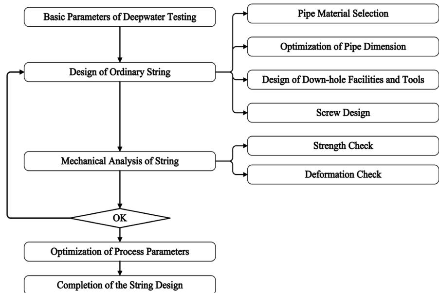
**Figure 1.** Optimization workflow of the string design in deepwater well testing.
