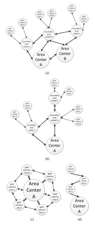
**Figure 3.** Visualization of boundary road structure and traffic flow. (a) Grid type; (b) tree type; (c) loop type; (d) linear type.
