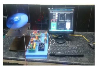
Figure 11. Experimental setup generator running condition with air blower.
