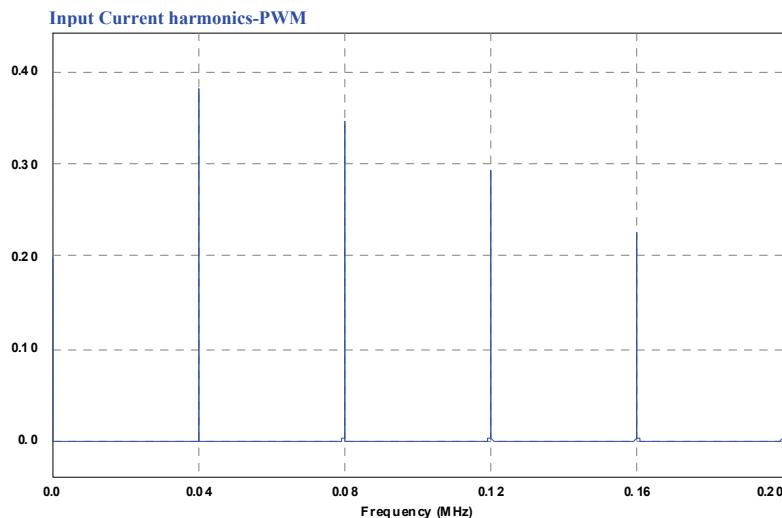
**Figure 8. Input current harmonic spectrum – PWM converter.**
