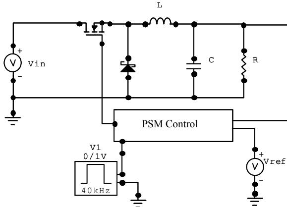
**Figure 1. Pulse skipping modulated buck converter.**
