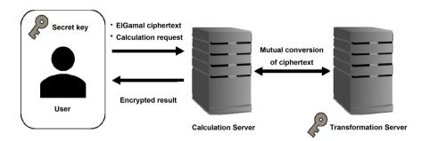
Figure 1. System configuration.
