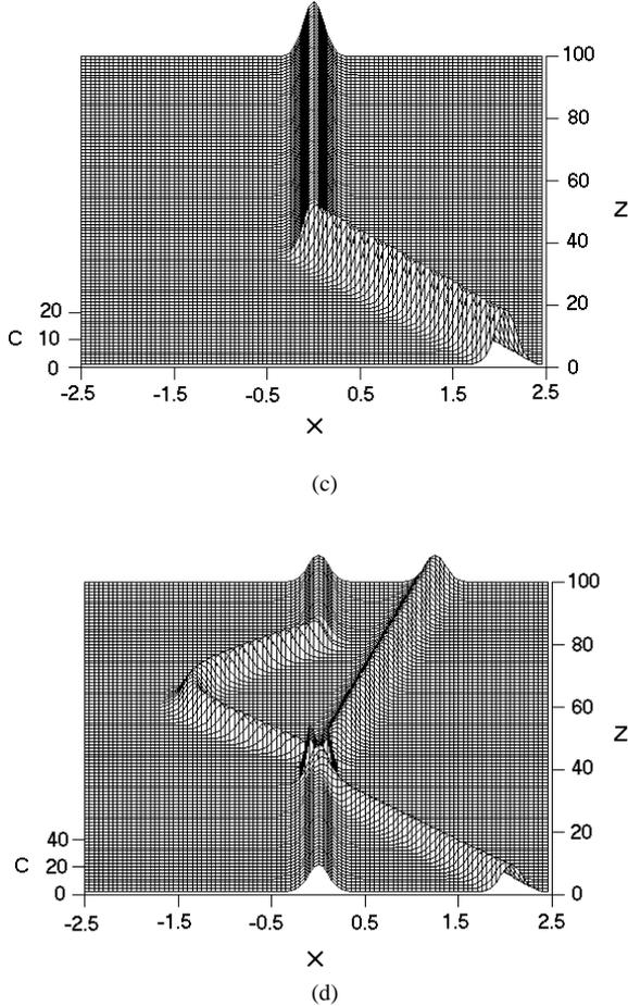
**Figures 6. Upper view and numerical simulations. The parameters of the waveguide are  $a=16.9$ ,  $d=1.4$ ,  $b=0.25$ ,  $\Delta n=1 \cdot 10^{-5}$ . (a) Upper view of the structure; (b) Numerical simulation of the behaviour of the structure in the presence of the only input 1; (c) Numerical simulation of the behaviour of the structure in the presence of the only input 2; (d) Numerical simulation of the behaviour of the structure in the presence of both input 1 and input 2.**
