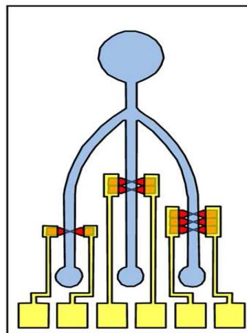
**Figure 2.** A lab-on-a-chip microfluidic device showing the inlet and outlets. (Source: Sharma *et al.*, 2013 [15]).
