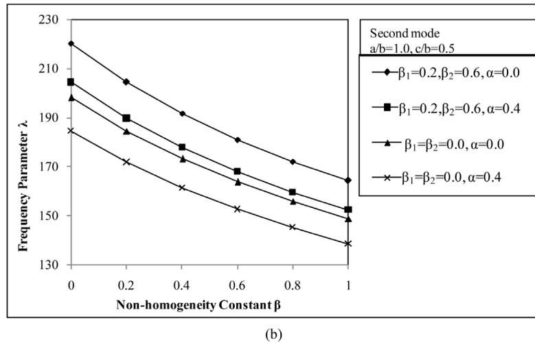
Figure 6. (a) & (b) Frequency parameter  $\lambda$  vs. non-homogeneity constant  $\beta$ .
