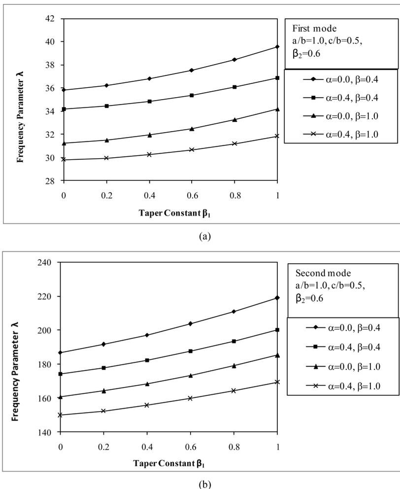
Figure 2. (a) & (b) Frequency parameter  $\lambda$  vs. taper constant  $\beta_1$ .
