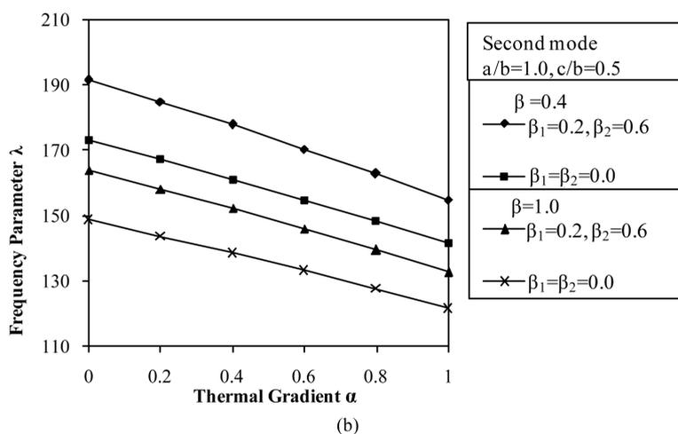
Figure 4. (a) & (b) Frequency parameter  $\lambda$  vs. thermal gradient  $\alpha$ .
