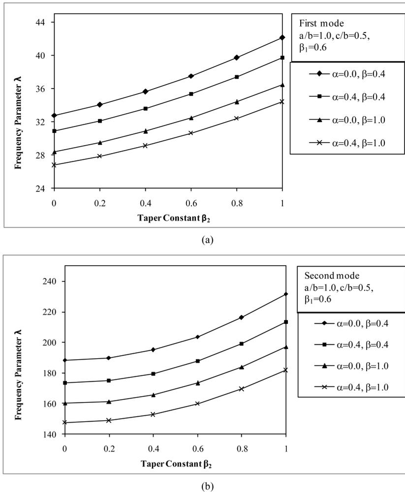
Figure 3. (a) & (b) Frequency parameter  $\lambda$  vs. taper constant  $\beta_2$ .
