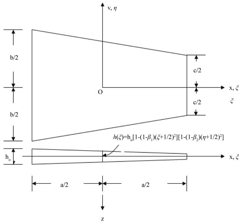
**Figure 1.** Geometry of the trapezoidal plate.
