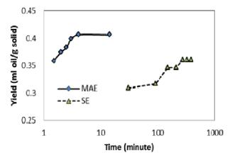
Figure 1. Comparison of soxhlet and microwave assisted extraction.
