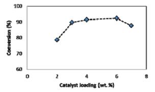
Figure 3. Effect of catalyst loading (Temperature 55°C, Methanol:Oil 4:1).
