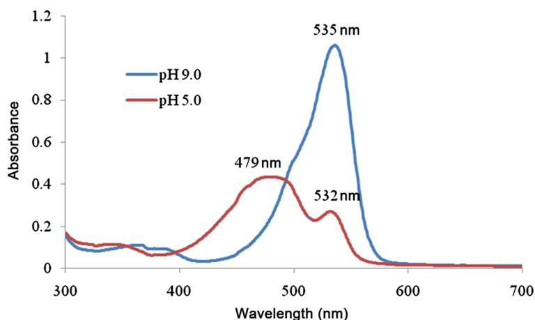
Figure 3. The UV-Vis spectrum of the pigment.
