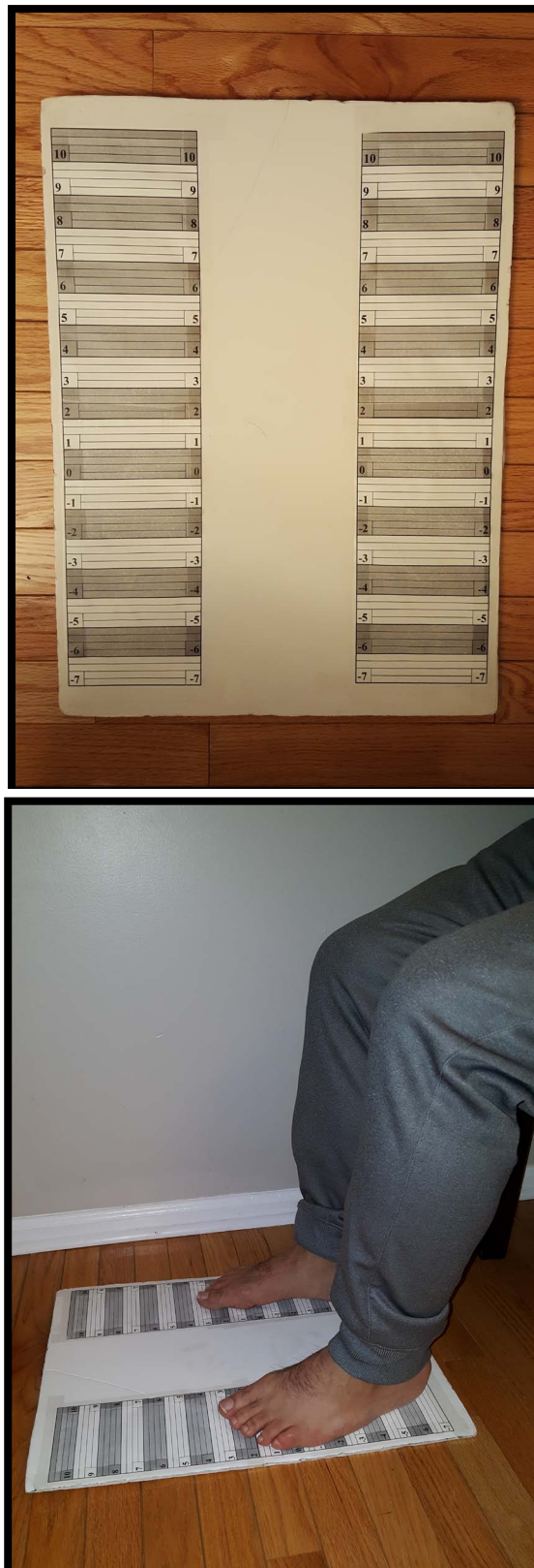
Figure 1. Kinesthetic Ruler designed to save time and efforts in the multiple measurements of the test or non-test legs movements during the kinesthetic awareness test-Procedure 2.
