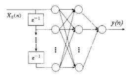
Figure 3. The secondary model based on the radial basis function neural network
