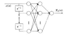
Figure 4. The controller of the active noise control based on RBF network
