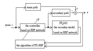
Figure 2. The model of the active noise control based on RBF network
