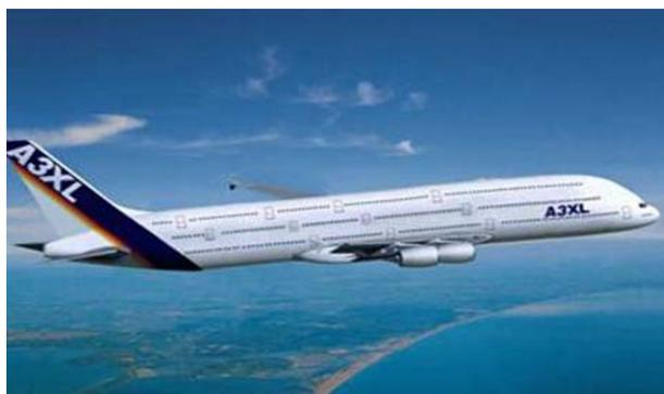
**Figure 5.** A sketch of a possible ultra high capacity aircraft for 1001 passengers. Source: H. J. K. Lemmen, modification of an Airbus website picture.
