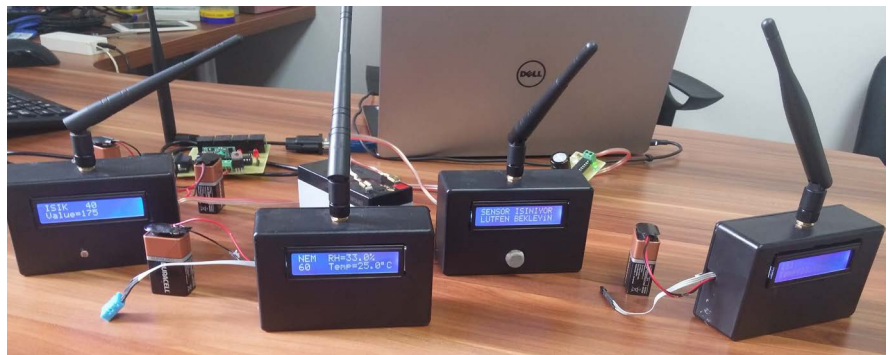
Figure 3. Overview of the designed WSN platform.
