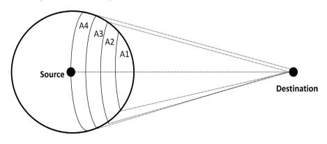
Figure 20. Priority region in GeRaF: increasing priority from A4 to A1 [70].
