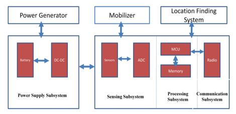
Figure 2. Architecture of a typical sensor node.
