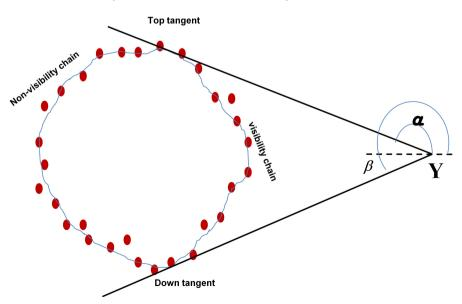
**Figure 26.** Visibility chain of a given node y consists of the nodes which are located between the two tangents and the destination.
