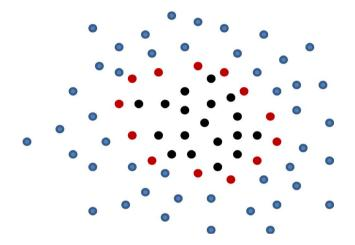
**Figure 25.** Network field containing the high loss region: Black nodes are lossy nodes, blue nodes are healthy nodes and red nodes are boundary nodes [85].
