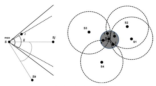
**Figure 23.**  $Ds = \{S1, S2, S3\}, D1 = \{S2, S3\}, D2 = \{S2, S1\}, D3 = \{S1\}, D4 = \{S3\}$ . The maximum allowed apex angle,  $a_{max}$ , and the apex of the shrink-est cone in the *Sj* direction that contain *i*, *ai*, *j*, are depicted [82].
