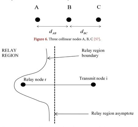
Figure 7. Relay region of the transmit-relay node pair in MECN [57].
