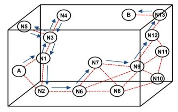
Figure 17. Example of LBRP routing a packet from node A to node B [65].
