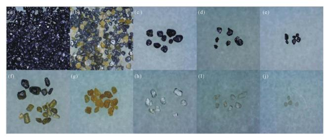
Figure 2. Microscope images of the magnetic part (a) which consists of magnetite and the non-magnetic part (b). The constituents of the non-magnetic part are hematite (c), ilmenite (d), allanite (e), diopsite (f), grossular (g), sanidine (h),  $\alpha$ -quartz (i), and calcite (j).
