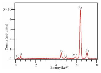
Figure 5. EDS spectrum of a magnetite grain with a partial substitution of Fe by Ti ( $\sim$ 6%) and Mn ( $\sim$ 2%).
