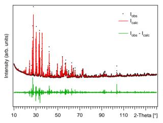
Figure 6. Powder XRD diagram of the non-magnetic part of the black sand. A pattern fitting (red line) shows the total contribution from eight phases. The composition of the nonmagnetic part was determined from Rietveld fits. The results are summarized in Table 2.
