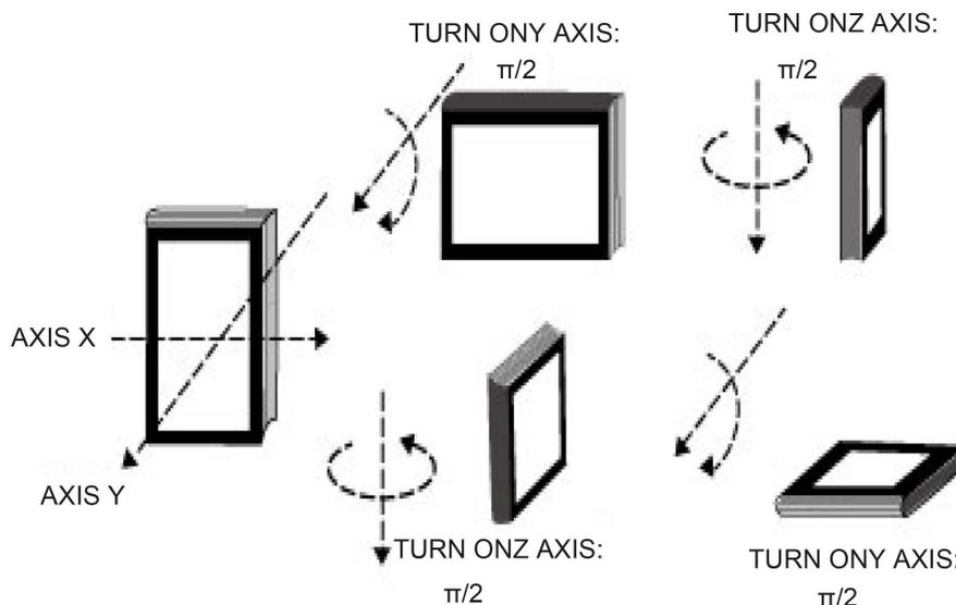
**Figure 7.** The result of two angular displacements referred to external axes differs depending on the order of application. The end position of the book is different after applying a quarter rotation on two different axes at different successive times [18].
