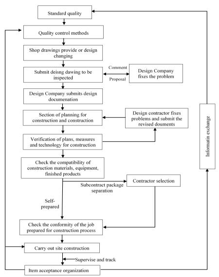
**Figure 2.** Diagram for quality control for construction of hydropower projecy in Vietnam.
