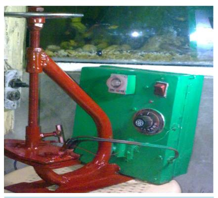
Figure 3. The portable electronic vulcanizer (PEV).
