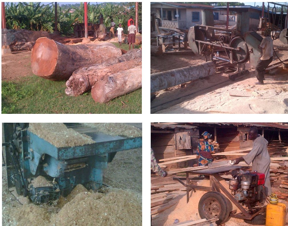
Figure 1. Typical activities such as debarking, canting, trimming and wood planing that generate wood waste in a Nigerian sawmill. Photos: Babafemi Oyebamiji.
