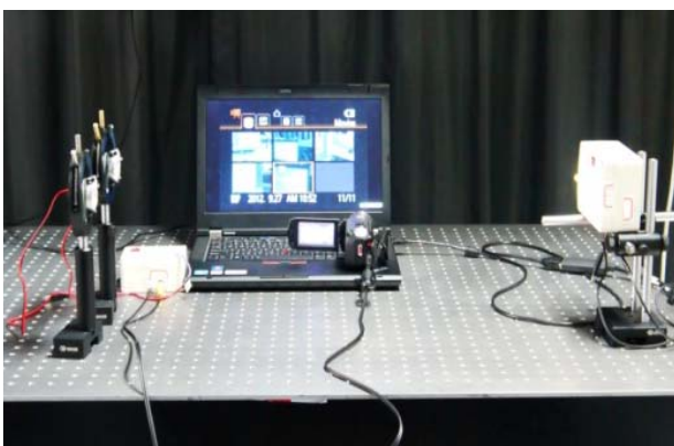
Figure 2. Picture of the real-time video/audio transmission prototype using LEDs.
