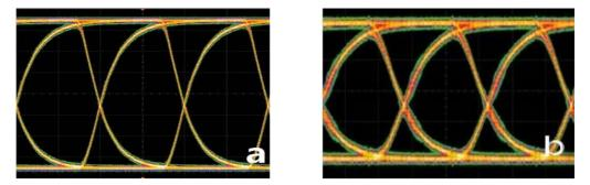
Figure 7. Eye diagram waveforms after direct detection without filtering and being amplified at (a) 1 Mbit/s data rate, (b) 2 Mbit/s data rate.
