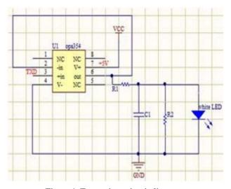
Figure 1. Transmitter circuit diagram.
