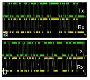
Figure 9. Captured data waveforms after decision circuit at (a) 1 Mbit/s data rate, (b) 2 Mbit/s data rate.
