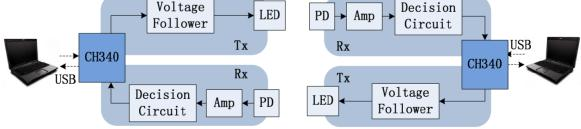
Figure 3. Transceiver block diagram.
